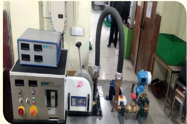
Turbine Supply Unit (Francis & Pelton)
