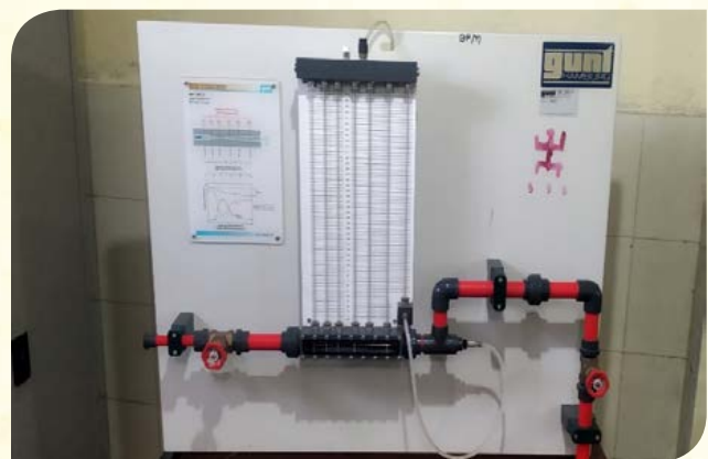
Bernoulli's Principle Demonstrator
