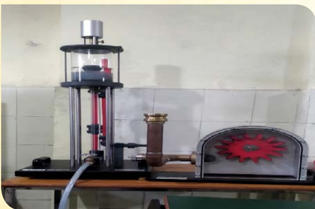
Reynold's Experiment Demonstrator
